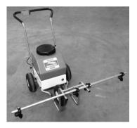
To remove the boom for storage and accessing narrow gateways by either releasing the 'D' clamps near front wheel and removing the boom sprayer assembly completely, or by reversing the first 3 steps mentioned above, and securing in place via the 'terry' clip on top of the 'S' bend.
