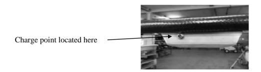
The battery charger is designed so that the battery can be left on charge until the machine is required. Although this will not damage the battery it is not recommended to do this very often.
